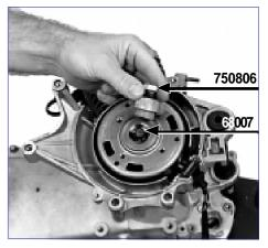
Screw the flywheel puller tool 750806 onto the rotor and tighten the centre bolt until the rotor comes away.
